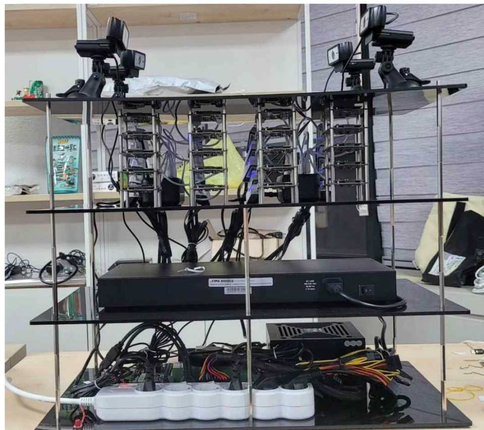
Figure 6. The hardware platform for multiple NPUs.
