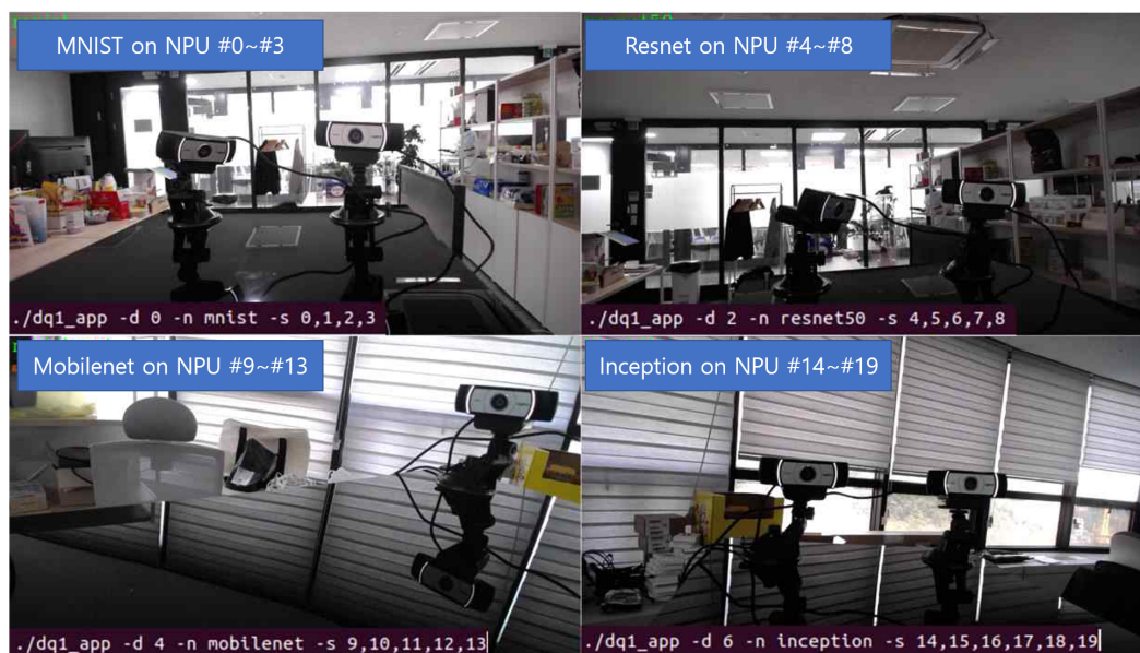
Figure 8. An example of inferring multiple DNNs on multiple NPUs.
