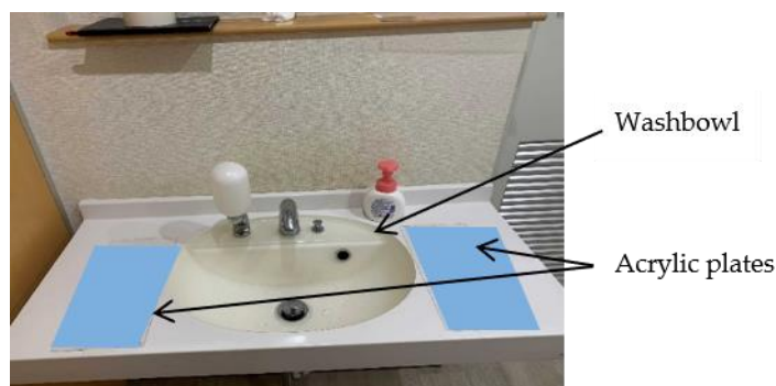
Figure 8. Photograph of the washbowl with acrylic plates placed on either side. Note that the acrylic plates, though transparent in the experiment, are shown in blue here for clarity.
