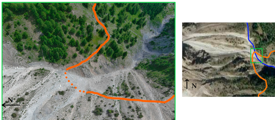
Figure 4. Drone photograph showing the Chaberton Military Road in orange and the ford, completely removed by the debris flow on 1 July 2019, with dashed lines. The panel on the right is located in the same position as the yellow square in Figure 1 and shows, in green, the position of the image on the left within the watershed. The blue line indicates the Rio Inferno.
