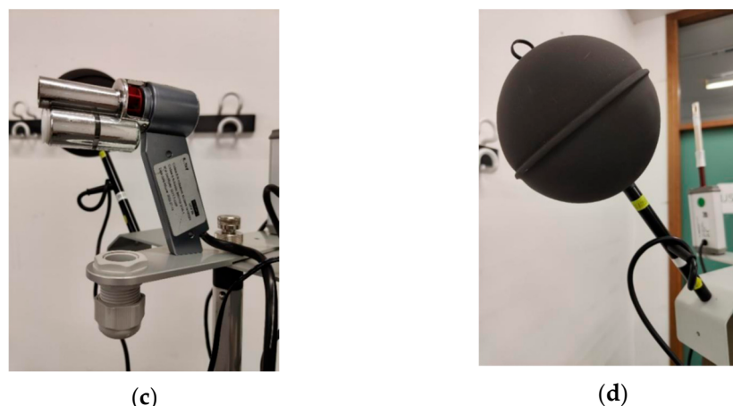
Figure 2. (a) overall BABUC system for microclimate assessment; (b) hot-wire anemometer; (c) psychrometer; and (d) globe thermometer.
