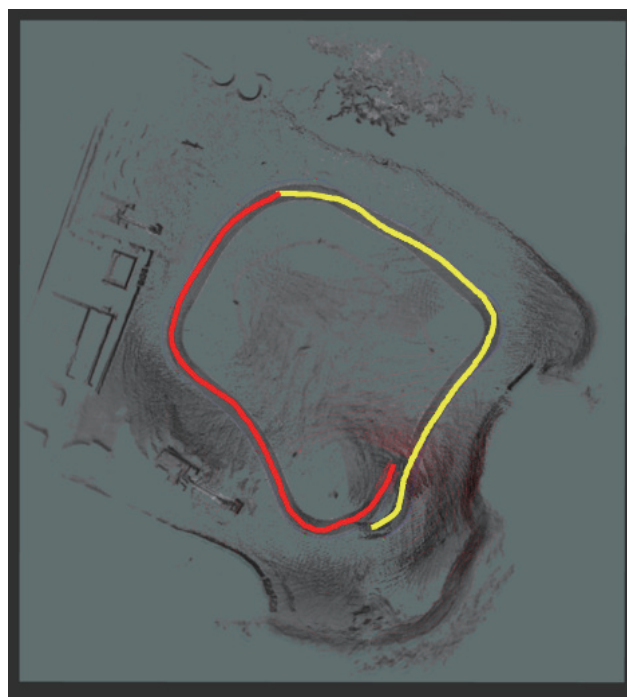
Figure 14. The result of multi-node SLAM execution. The yellow and red lines represent the SLAM execution routes for bag4_split_1 and bag4_split_2, respectively.
