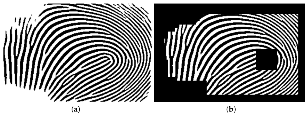
Figure 14. A sample binarized image from Figure 3a is shown in (a), and its quality-mapped image, which only includes the highest-quality sections of the binarized image (quality 4), is shown in (b).
