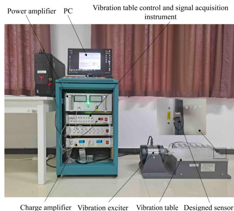
Figure 14. Physical diagram of sensor vibration signal test device.
