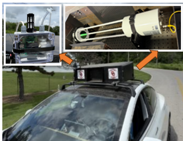
Figure 9. Driving Test Setup: The left panel shows the AIMNet sensor mounted on the mobile test platform, while the right panel displays the LI-COR 7700 reference instrument used for performance comparison.
