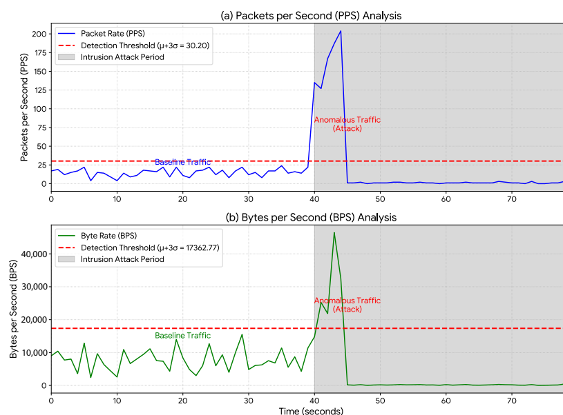
Figure 6. Intrusion Attack Detection Using PPS and BPS Metrics. Results from the intrusion attack simulation (shaded region, t \geq 40 s). The attack produces a distinct, short-duration traffic spike that markedly exceeds the \mu + 3\sigma statistical baseline (red dashed line) for both (a) Packets per Second (PPS) and (b) Bytes per Second (BPS). This clear threshold violation confirms the method's capability to identify unauthorized intrusion events based on their data-rate footprint.
