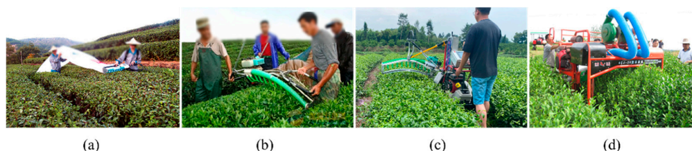
Figure 1. Structures of tea plucking machine: (a) single hand-held, (b) double-carried, (c) self-propelled and (d) track riding type.
