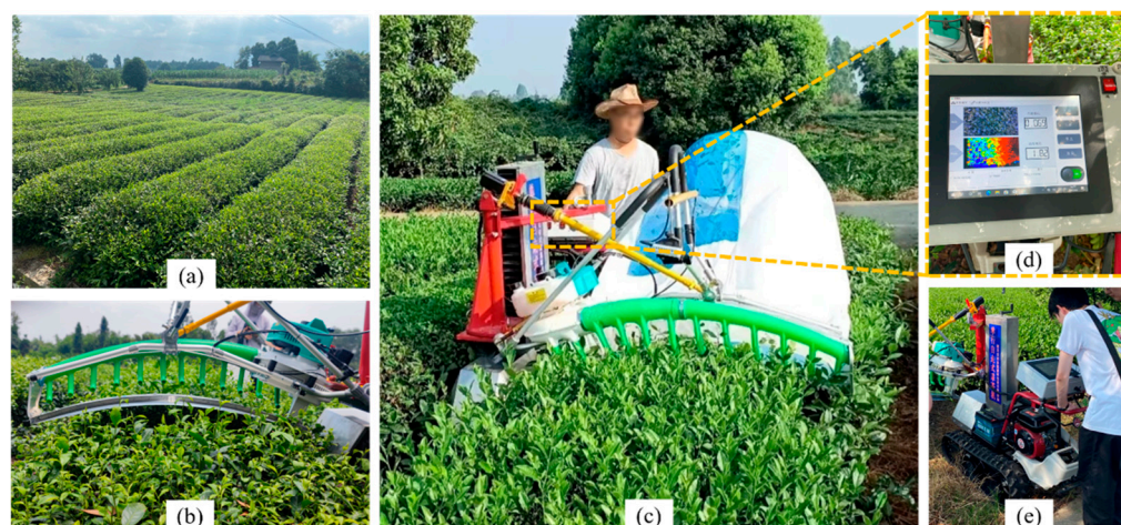
Figure 3. Bulk tea plucking system: (a) experimental tea plantation used in this study, (b) the arch-shaped cutter and tea canopy, (c) the tea plucking machine with an operator, (d) human-machine interface, and (e) the crawler chassis.
