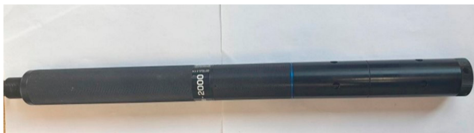
Figure 3. The AquaSond-2000 (AS-2000) multiparameter water quality monitoring sonde used for continuous monitoring during the study period.
