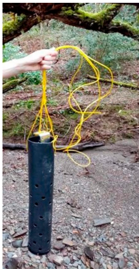
Figure 4. Deployment setup of the AS-2000 within a protective plastic housing that allowed water to flow freely past the sensors while shielding the device from damage due to debris or sediment build-up. The sonde was anchored at a fixed point to ensure consistent submersion and was routinely checked to ensure continued operation and data quality.
