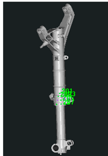
Figure 5. Transformation of Key Points from Close-Range Photogrammetry to the Measurement Coordinate System.
