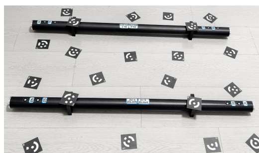
Figure 10. Verification of the accuracy of the close-range photogrammetry system.
