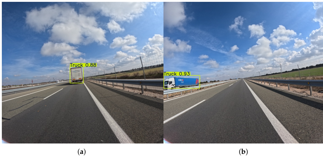
Figure 14. Representative outputs of the YOLOv8s model with an input size of 1120 \times 1280 , which demonstrates the best overall performance in the truck detection task. An example (a) demonstrating successful detection of a truck in an adjacent lane, shown at a moderate distance, and (b) showing accurate detection of a distant truck.
