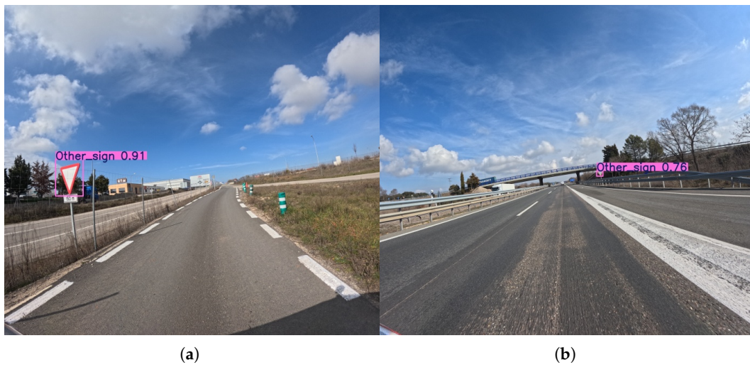
Figure 12. Representative outputs of the YOLOv8l model with an input size of 1120 \times 1280 , which demonstrates the best overall performance in the other sign detection task. An example (a) demonstrating successful detection of a sign on a low-speed access road adjacent to an industrial area, and (b) showing detection performance on a sign positioned on the side of the highway.
