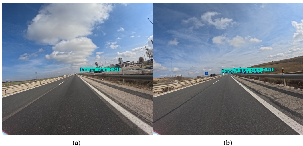
Figure 10. Representative outputs of the YOLOv8l model with an input size of 1120 \times 1280 , which demonstrates the best overall performance in the danger sign detection task. An example (a) demonstrating successful detection of a Danger sign positioned close to the roadside guardrail, and (b) showing detection of multiple Danger signs with a different background.
