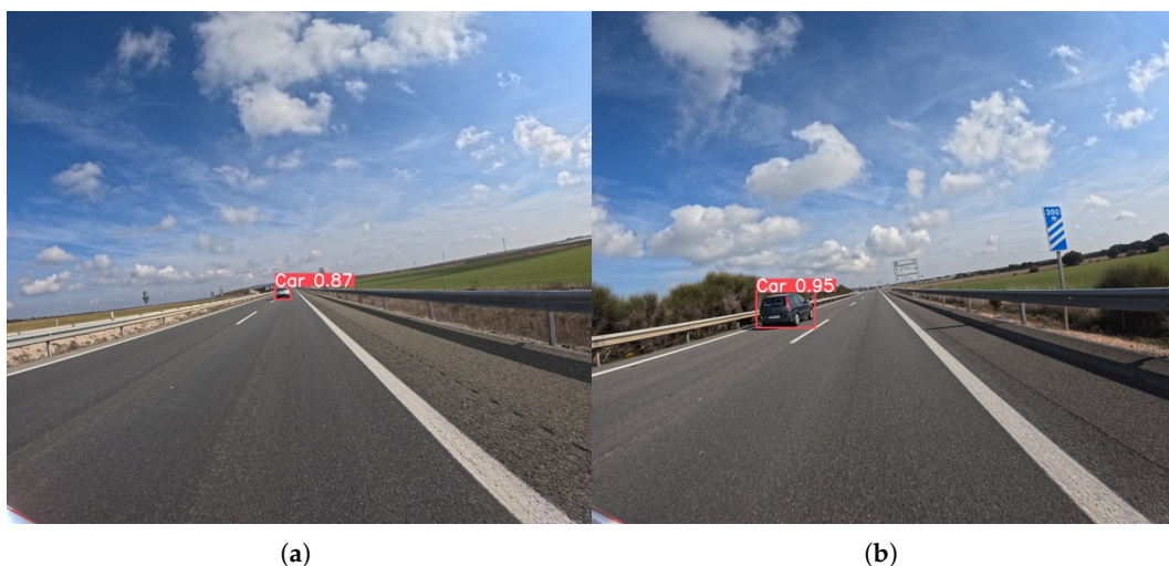
Figure 13. Representative outputs of the YOLOv8l model with an input size of 1120 \times 1280 , which demonstrates the best overall performance in the car detection task. An example (a) demonstrating successful detection of a distant car, and (b) showing accurate detection of a closer car on the highway.
