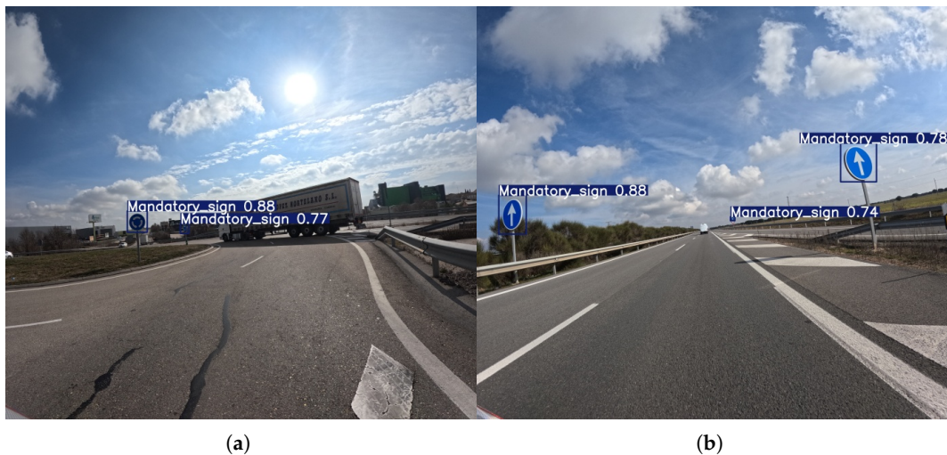
Figure 11. Representative outputs of the YOLOv8m model with an input size of 1120 \times 1280 , which demonstrates the best overall performance in the mandatory sign detection task. An example (a) demonstrating successful detection of Mandatory signs in a complex scenario involving sun glare and occluding vehicles (truck), and (b) showing detection performance on several Mandatory signs positioned at different distances on an open highway.
