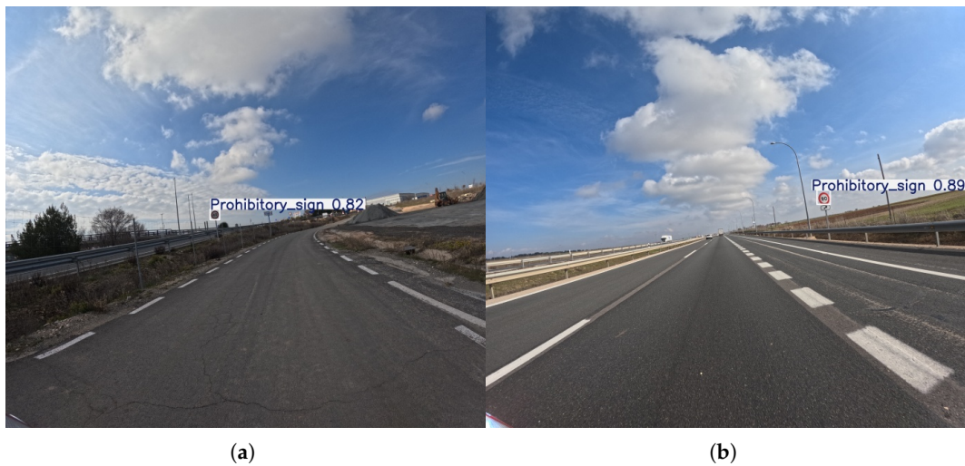
Figure 9. Representative outputs of the YOLOv8l model with an input size of 1120 \times 1280 , which demonstrates the best performance in the prohibitory sign detection task. An example (a) showing detection of a sign on an access road, and (b) showing detection of a speed limit sign on a highway.
