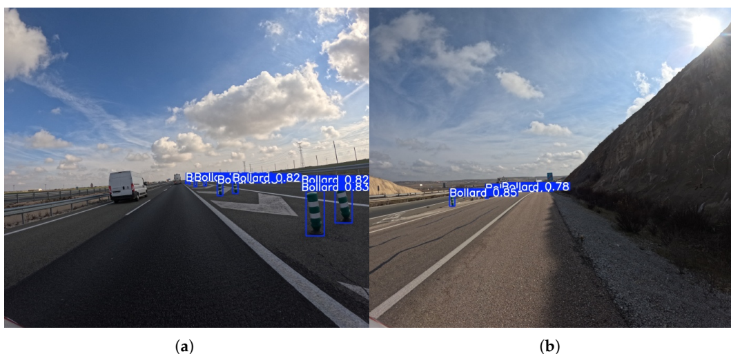
Figure 7. Representative outputs of the YOLOv11l model with an input size of 1120 \times 1280 , which demonstrates the best overall performance in the bollard detection task. An example (a) demonstrating successful detection of multiple bollards on a high-speed road, and (b) showing detection of bollards in a challenging low-light/high-contrast roadside environment.
