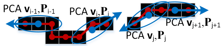
Figure 3. The end curve models are PCAs constructed from the first n^{pts} and last n^{pts} pixels of each curve (shown as blue ellipses) and aligned to point outwards from the curve.
