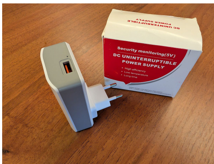
Figure 3. Uninterruptible power supply for AIR811 sensors: input, 220 V/0.5 A; output 5 V/2 A. Sensor operation time up to 30 min (measured in practical testing).
