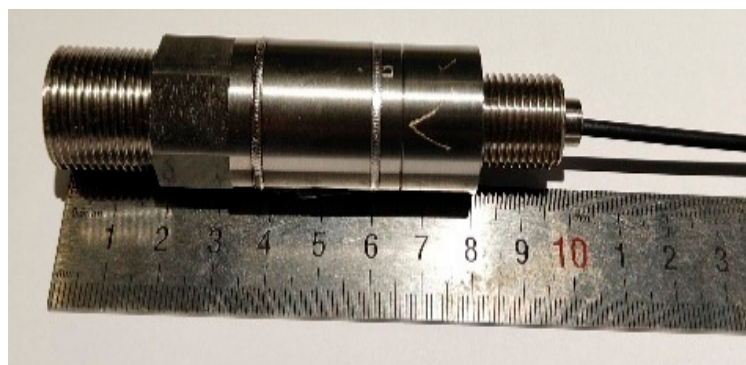
Figure 7. Overall diagram of the sensor. Each pure metal shell module is assembled and laser welded, with a length of 10 cm.
