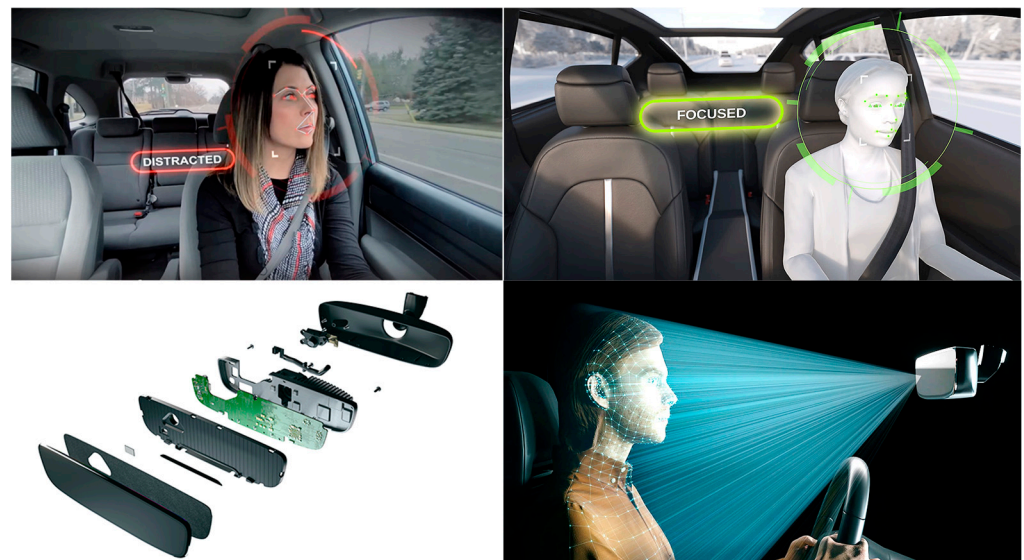
Figure 20. Key features of Magna DMS: distracted driver detection, drowsy detection, occupant detection, child presence/seat detection, occupant classification, properly worn seatbelt detection.
