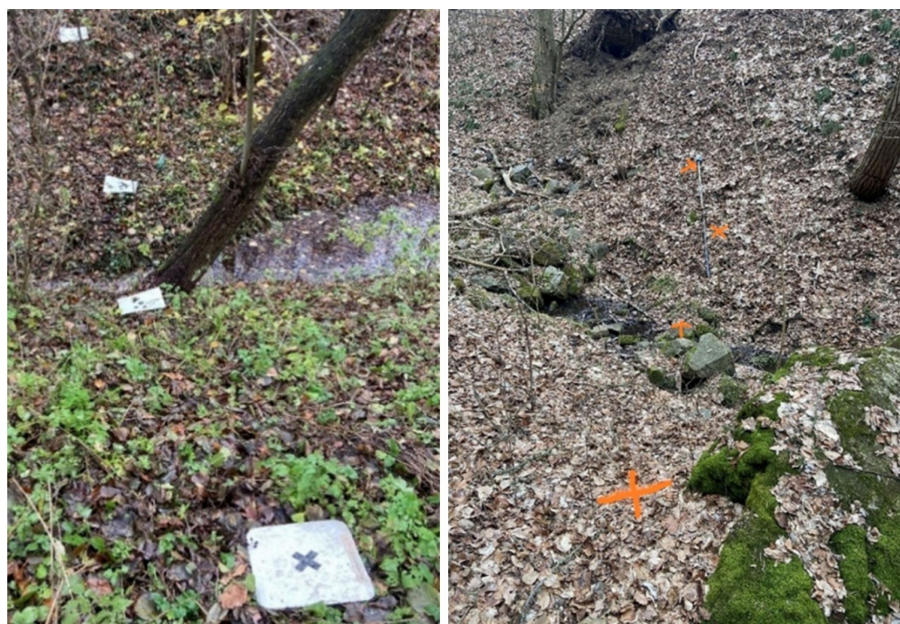
Figure 4. (Left)—Cross profile with marked reference points (plastic and metal target), (Right)—spray painted markers for sectional scanning (orange spray paint).
