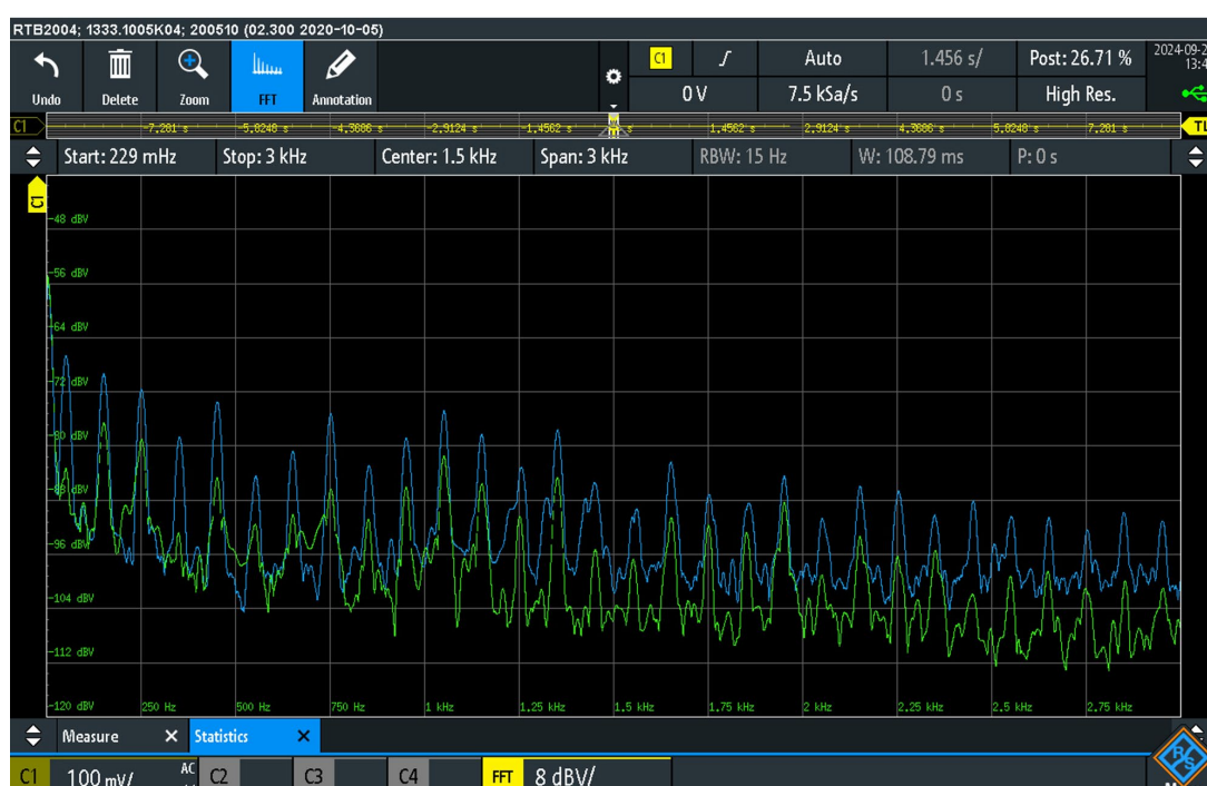
Figure 6. Spectral measurements of the influence of ground loop termination on the EMI: Blue—non-terminated loop, green—terminated loop.
