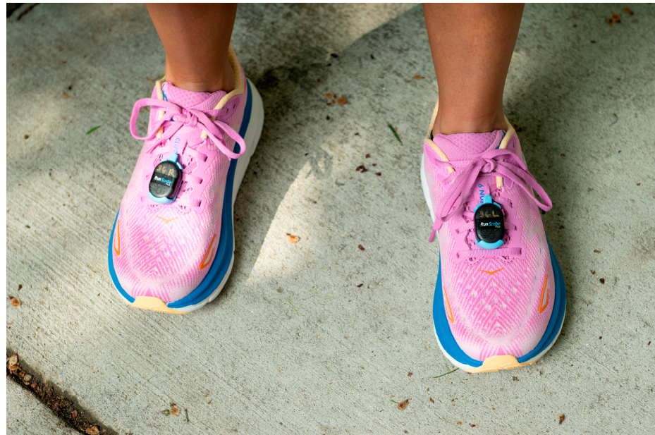
Figure 1. Image showing placement of bilateral lace-mounted IMUs, secured with the specific lace cradles at the midfoot of the running shoes.
