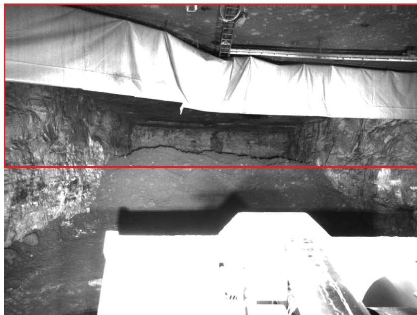
Figure 3. Example image taken from the left camera. The red rectangle shows the area that is set to half intensity on average by controlling the exposure time and the gain. The bright bucket is overexposed due to this optimization, but the environment is easily recognizable.
