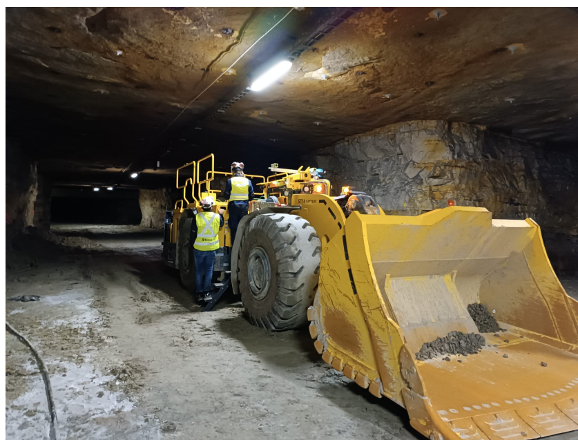
Figure 5. ST14 used for testing the muck pile detection system.
