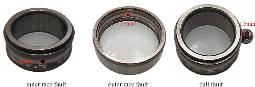
Figure 6. Three types of bearing failure conditions at a damage level of 1.5 mm.
