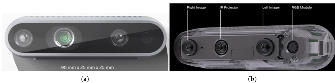
Figure 4. Intel RealSense camera views: (a) Outer view. (b) Inner view.
