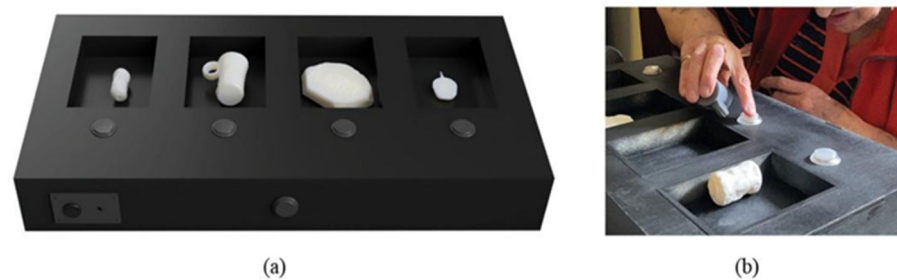
Figure 2. The Writing and Pushbuttons ITUI: (a) The ITUI comprises four items: (right to left) charm, legion tile, inkwell, and cylinder seal. (b) A Pushbutton is positioned in front of every box corresponding to the piece.
