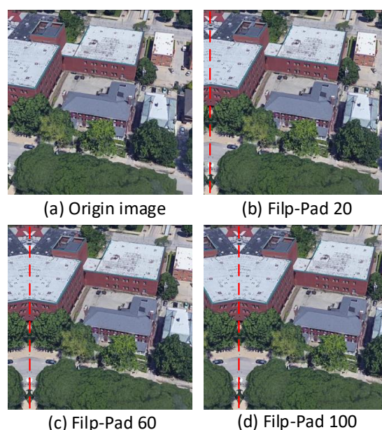
Figure 6. Illustration of mirror padding. The rightmost part of the image is cropped, and the leftmost region of the same width is mirrored to the left to maintain the original image size. (a) Original drone image; (b) left-side mirror padding of 20 pixels; (c) left-side mirror padding of 60 pixels; (d) left-side mirror padding of 100 pixels.
