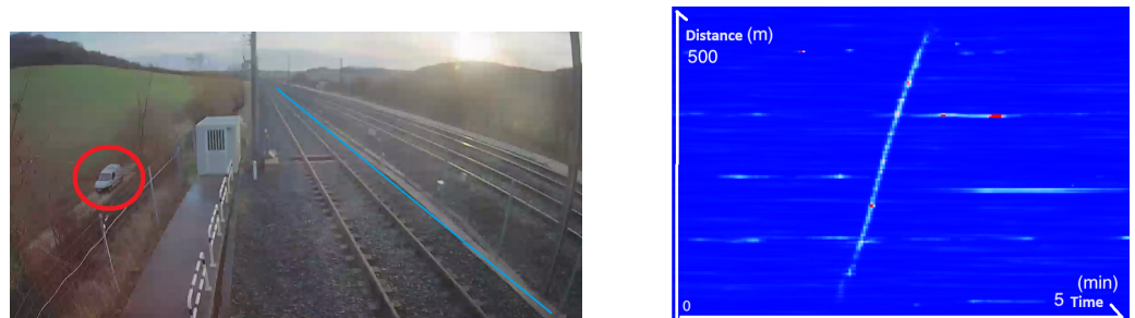
Figure 3. Left: Image taken from a CCTV camera showing the car driving past the railway line. The car is surrounded by a red circle, and the location of the fiber is indicated by a blue line. Right: The associated frequency band energy between 0 and 250 Hz showing the movement of the car.
