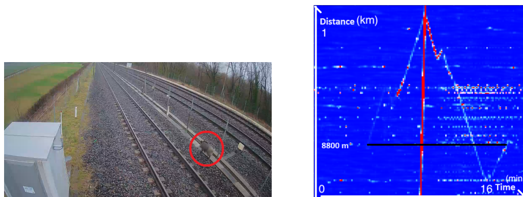
Figure 7. Left: Image taken from a CCTV camera showing the wild boar (red circle). Right: The associated frequency band energy between 0 and 250 Hz showing the boar trajectory.
