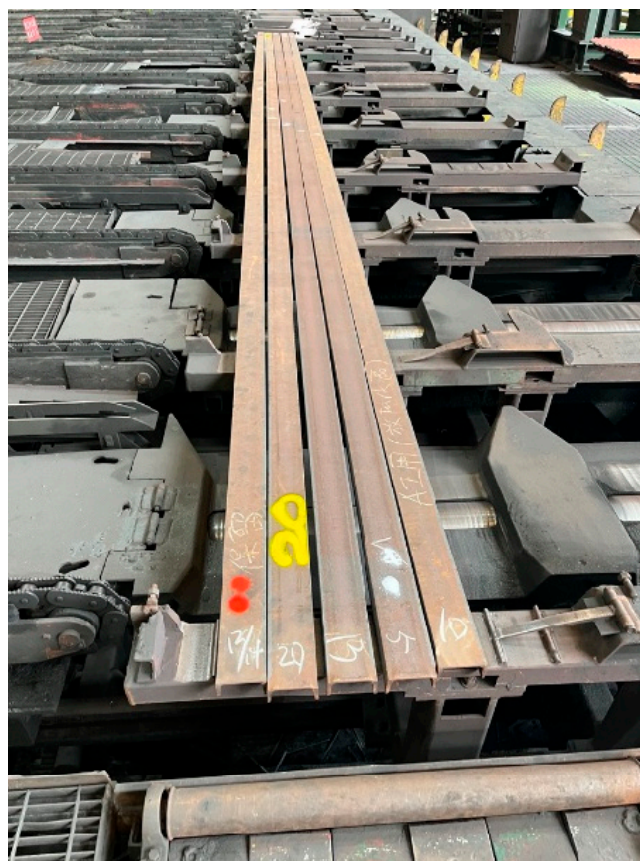
Figure 2. Sample steel bars used for establishing inspection standards. (There are some Chinese words on the steel bars such as “保留” and “AI用”, which mean “Reserved” and “Used for the AI field”, respectively).
