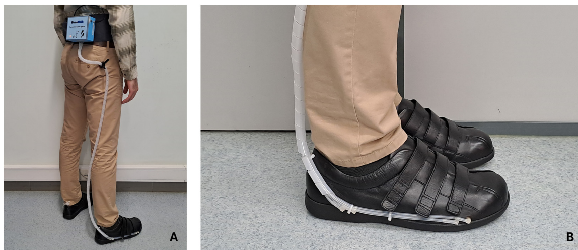
Figure 8. User equipped with the variable pressure system: (A) pneumatic control unit attached to the waist; (B) final appearance of the shoe (Ortomedical, Doctor Karl, EU44) with pneumatic insole.
