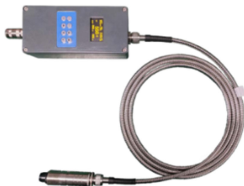
Figure 5. A physical picture of the colorimetric thermometer.
