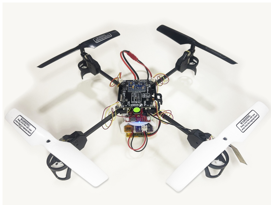
Figure 11. A quad-rotor UAV with RUL LiPo battery-embedded AI sensor.
