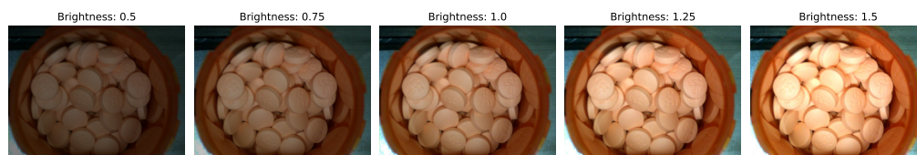
Figure 3. Effects of varying brightness factors (from 0.5 to 1.5) on a sample waste image used to simulate lighting condition changes for robustness testing.
