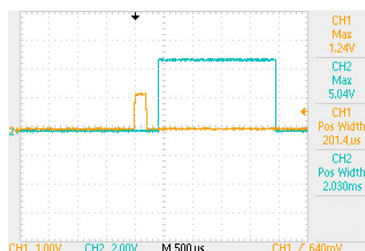
Figure 4. Synchronization of data acquisition with the stimulation. In orange, the signal detected at the electrodes (for 1 mA). In blue, the trigger applied to the EEG amplifier.
