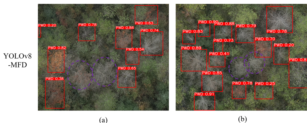
Figure 12. Examples of missed detections for dead-stage trees with white branches. Subfigures (a,b) show typical false negative cases, where clusters of closely adjacent trees in the death stage were not detected by the model. Dashed purple circles indicate the undetected regions.
