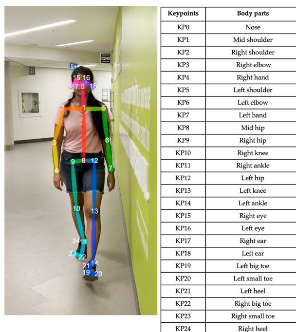
Figure 3. OpenPose human pose estimation using BODY25 model [22].
