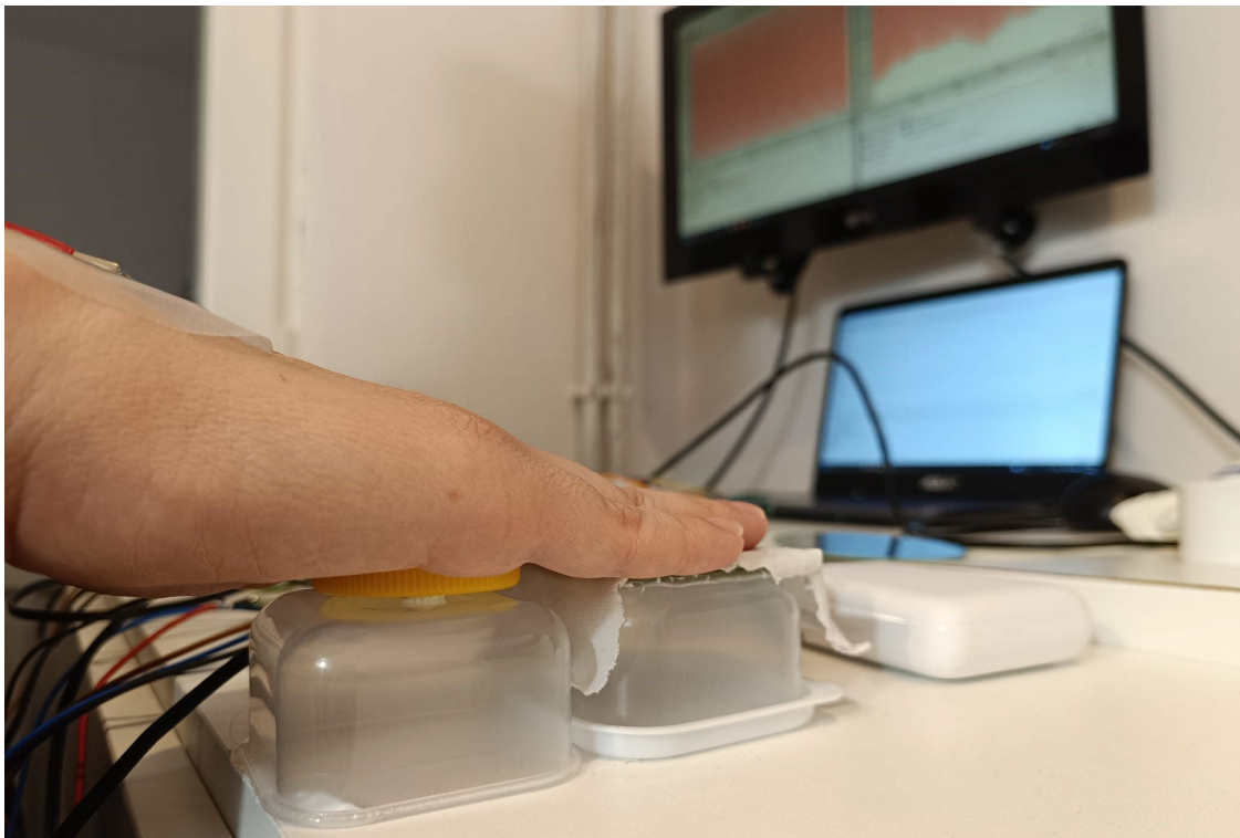
Figure 7. Placement of hands over the sensors and non-contact electrodes mounted on the plastic mounts (shown in Figure 6).
