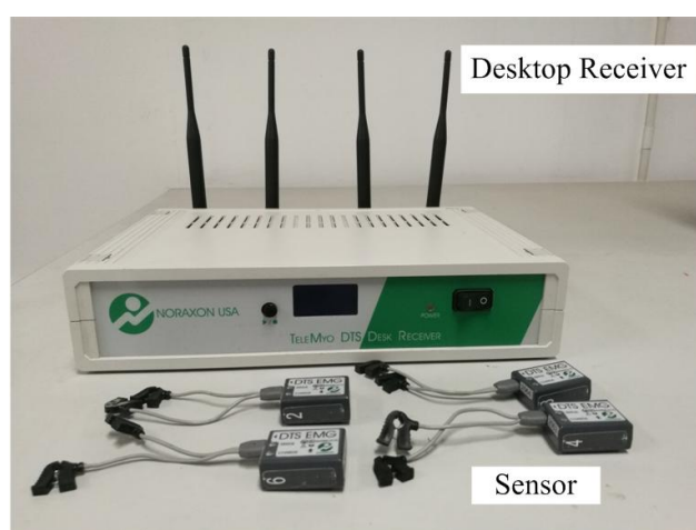
Figure 3. Wireless sEMG acquisition device used in the experiment.
