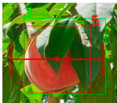
Figure 6. The example image of gripping success. Green boxes are ground truth and red boxes are predictions. The grip is generated with \alpha = 20\% .
