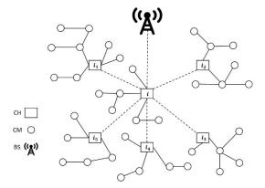
**Figure 7.** Inter-cluster trust configuration where CH *i* is directly engaging with CHs *i*1, *i*2, *i*3, *i*4, and *i*5.
