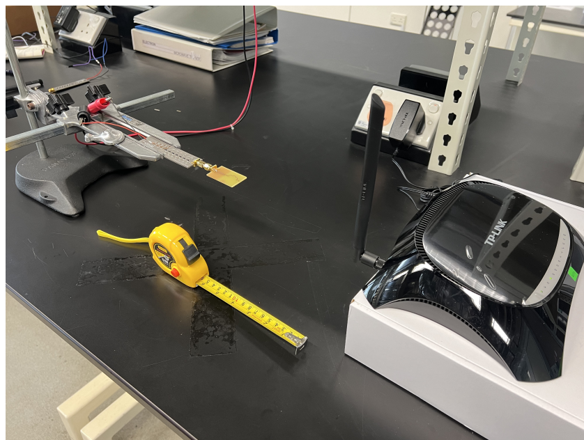
Figure 19. DC output voltage measurement of rectenna system with Wi-Fi router as RF source.
