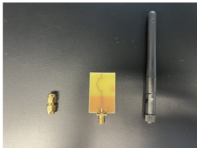
Figure 17. A male-to-male SMA connector jack, fractal antenna, and 2.5 dBi dipole antenna used for testing.
