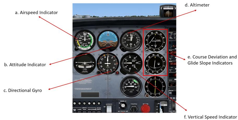
Figure 2. The Cessna 172 Steam Gauge (SG) panel.
