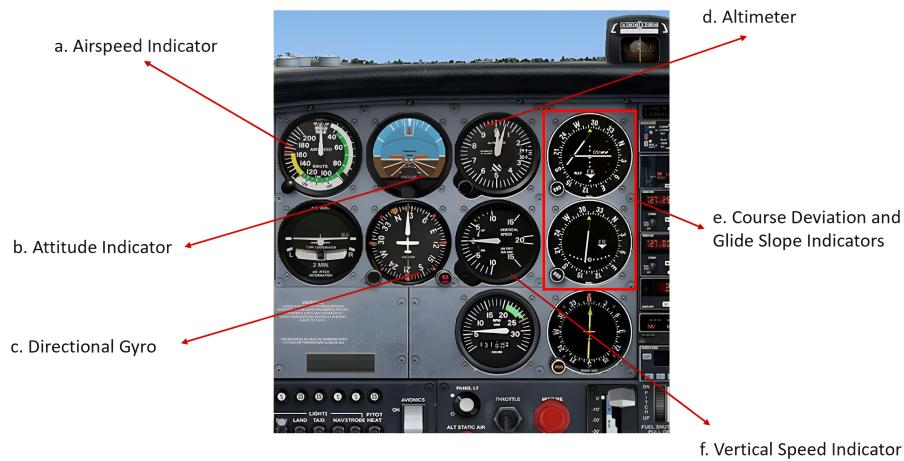
**Figure 2.** The Cessna 172 Steam Gauge (SG) panel.
