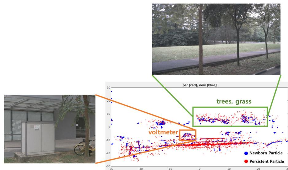
**Figure 3.** Persistent and newborn particle distribution of LiDAR-based DOGM.
