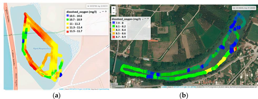
**Figure 6.** Dissolved Oxygen by the Waquin application of INTCATCH in (a) Koumoundourou Lake and (b) Acheloos river.
