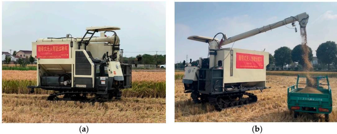
**Figure 19.** Platform and environment of the trials: (a) Experiment environment for automated navigation; (b) Experiment site for automatic grain unloading.
