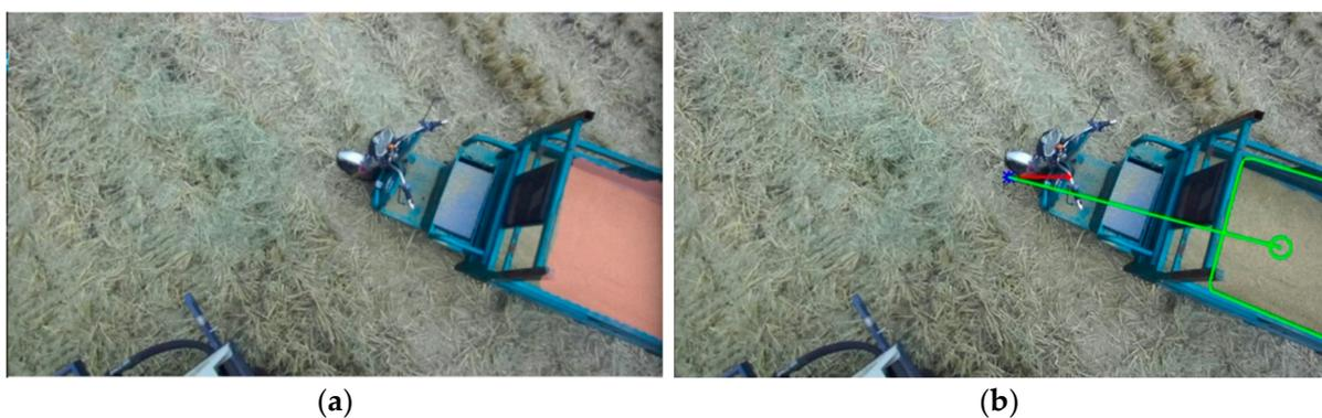
**Figure 15.** Fitted rectangle of the incomplete unloading area: (a) Semantic segmentation effect; (b) Fitted rectangle effect.
