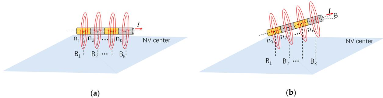
**Figure 2.** (a) Angle measurement based on the magnetic field when the wire is parallel to the diamond; (b) angle measurement based on the magnetic field when there is an angle  $\theta$  between the wire and diamond.
