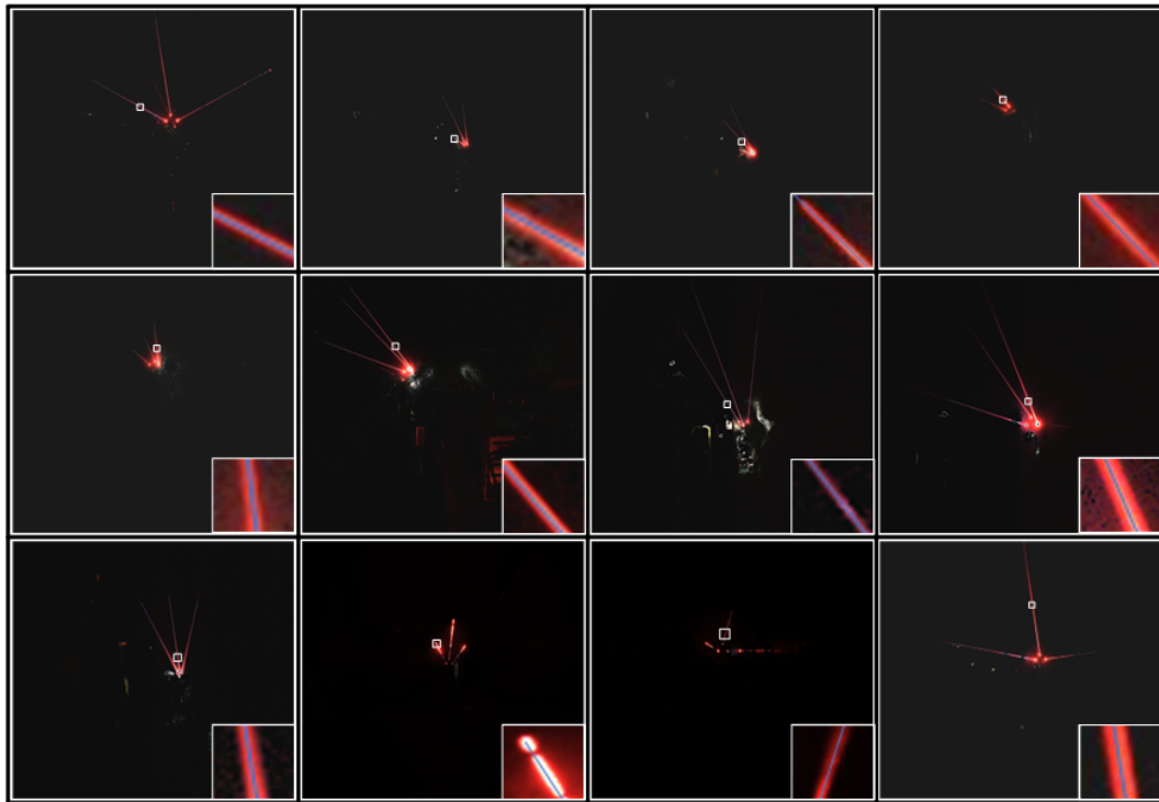
Figure 14. The center line fitting results of multi-laser beams.
