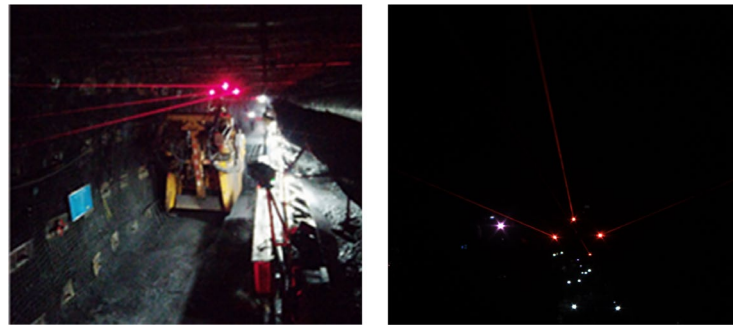
Figure 1. The laser beam-based visual positioning system that was under industrial testing at the tunneling face and its collected laser beam image.
