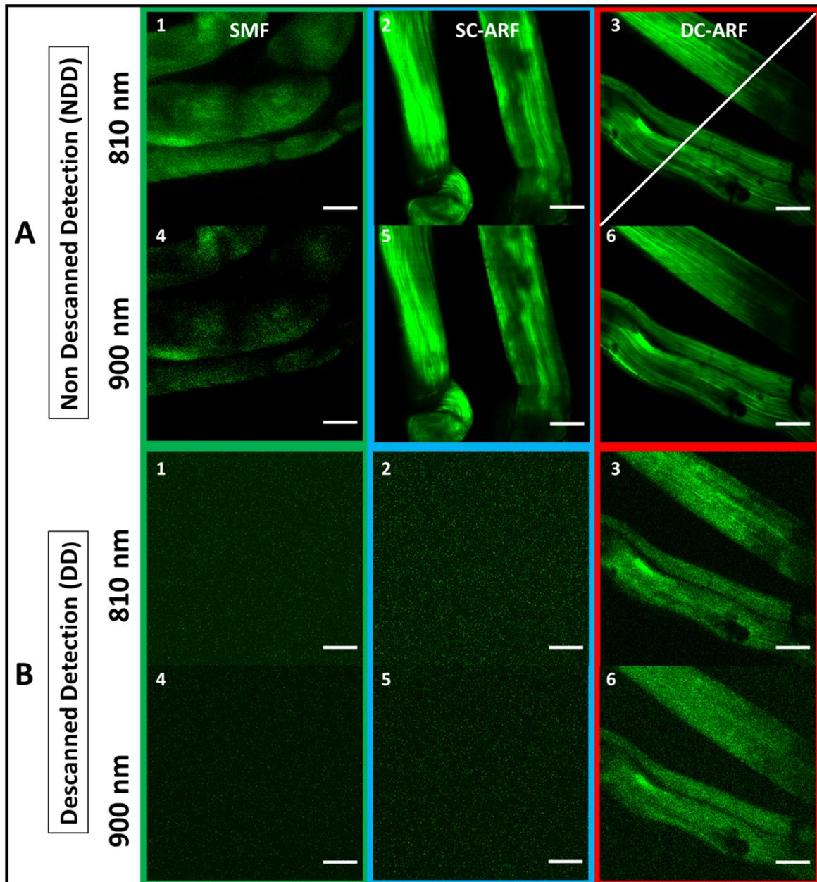
**Figure 4.** SHG imaging of biological samples with all fibers. The corresponding images of mouse tail tendon taken using NDD (A) (1–6), and DD (B) (1–6) configuration for a 3 m long SCF, SC-ARF, and DC-ARF at 810 nm and 900 nm excitation wavelength are shown; (NDD: 20× objective, zoom 3, 341 pixels, 10.7  $\mu$ s dwell time, ~20 mW power; DD: 20× objective, zoom 3, 341 pixels, 27  $\mu$ s dwell time, ~20 mW power, average 10 frames). Scale bar = 50  $\mu$ m.
