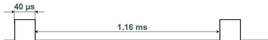
Figure 10. Laser pulse timing characteristic.
