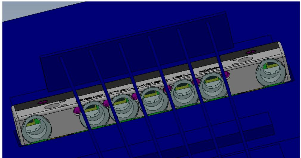
**Figure 5.** Design of the mechanical mounting for seven PSDs and six lasers.
