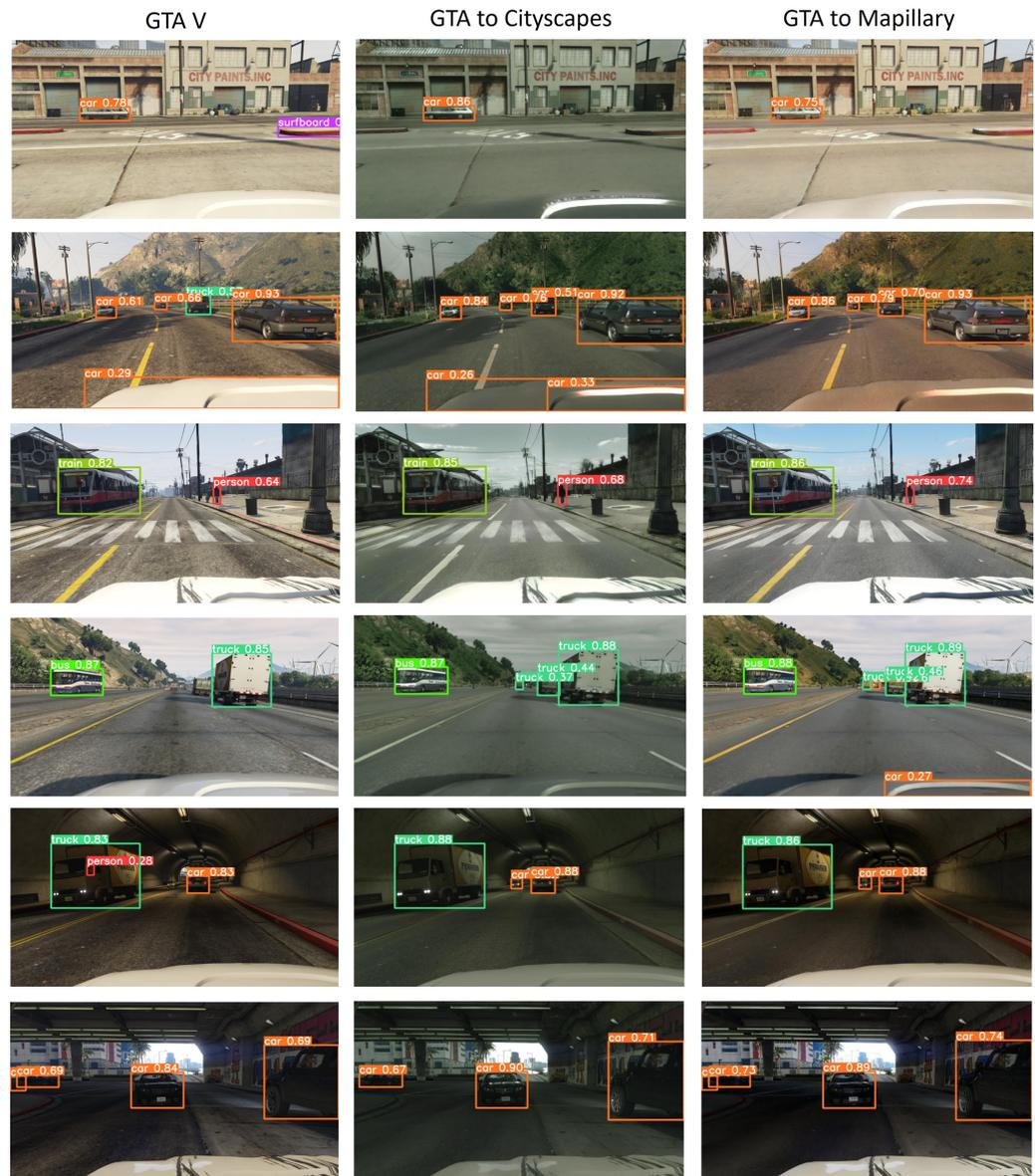
**Figure 9.** Example of object detection with the YOLOv5 algorithm applied to GTA V and enhanced GTA images.
