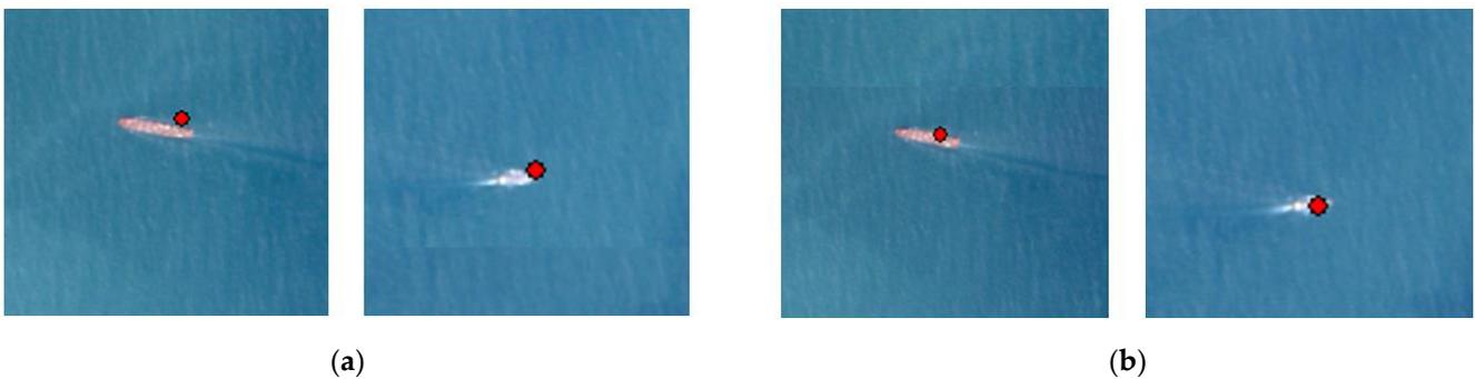
**Figure 16.** Display of correspondence between the remote-sensing image and the AIS data before and after positioning error correction. (a) Before positioning error correction; (b) after positioning error correction.
